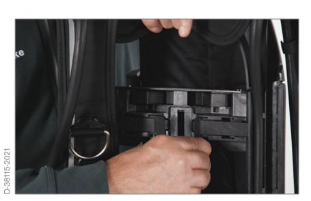
For height adjustment of the backplate, lift equipment into vertical position. Release yoke by depressing the buttons. Adjust yoke to required torso length. Ensure the buttons are in the locked position following setting.
