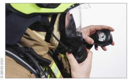
Connect LDV to the full face mask. Breath normally while monitoring the gauge. Once the gauge shows 60 to 50 bar the low pressure warning whistle will sound. Continue breathing until the pressure gauge shows 0 bar. Inhale and hold your breath. There must be no noticeable air ingress, otherwise check the mask fit.
