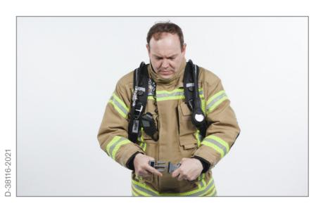
To don the SCBA, put the carrying system on one shoulder first, followed by the other. Close the buckle of the waistbelt and pull, ensuring the set sits comfortably on your hips. Tighten the shoulder straps, leaving a space between the shoulder and the harness to allow freedom of movement.
