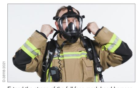
Extend the straps of the full-face mask head harness. Place the chin part of the mask at your face, then gently push onto your face and adjust it by pulling the lower strap straight back first and pulling the upper straps afterwards. Ensure that the middle strap is centered at the top of your head.
