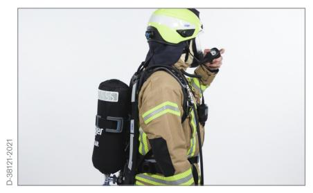
During pressurization, a momentary sounding of the whistle will occur. Fully close the cylinder valve. After one minute, check the gauge. It should show a pressure drop of less than 10 bar.
