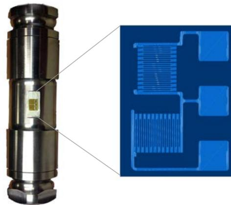
Shown here is the internal column of a compression load cell, sometimes referred to as a canister load cell, noting the placement of the strain gauge(s). As load is applied to the scale, the column compresses, which changes the electrical output of the strain gauge to measure weight.
