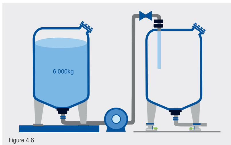
A known weight is being transferred from one scale (the reference scale) to the tank scale to be calibrated
