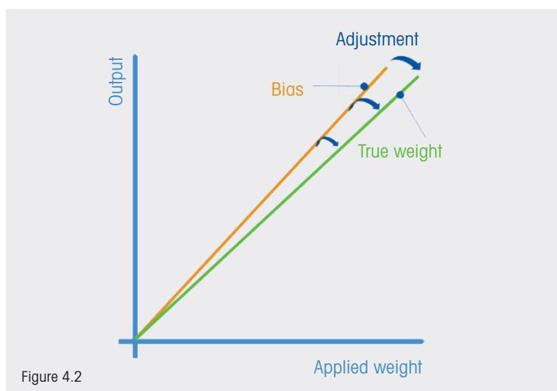
Weightless calibration can adjust the slope of the sensitivity to a more ideal position but is not considered a calibration
